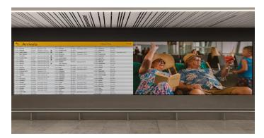
In comparing a 1.2mm and 1.5mm pixel pitch side by side, after a period of evaluation the team at Brussels Airport selected the LED-FE012i2 product with a finer pixel pitch ensuring the clarity and readability of flight information from close distance.
